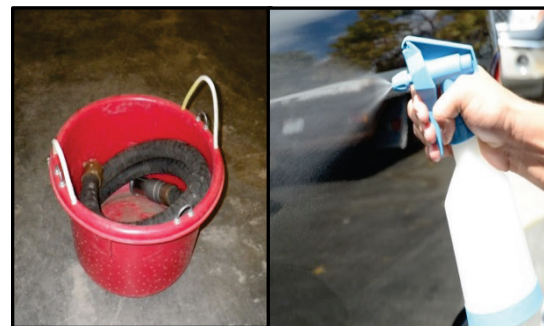
Figure 5. If drying or hot water are not options, draft hoses with foot valves can be decontaminated by submerging in a bucket filled with disinfectant. Alternatively, disinfectant can be sprayed on.
