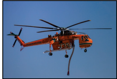
Figure 6. Helicopter snorkels, such as on this Sky Crane, do not need priming so no risk of tank water leakage during drafting. However, snorkel ends and foot valves that touch untreated water must still be decontaminated.
