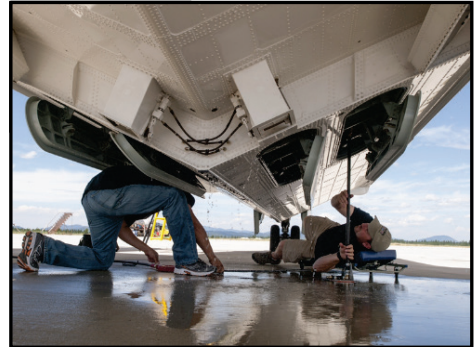
Figure 7. A CL-415 scooper plane fills its belly tanks [inset]. Workers decontaminate belly tanks of CL-415 scooper plane by spraying hot water from a high pressure wand and a portable hot washer, or ‘Hotsy’.
