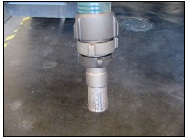
Figure 9. Foot valve attached to suction line with various adapters as needed to adjust for foot valve size.
